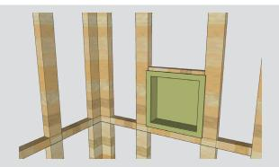
Step 2: Dry fit the niche into the framed cavity to check for size.
