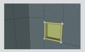
Step 5: Pre-Drill then, Screw in a minimum of 4 small countersunk stainless steel screws and washers through the flange to hold firm. Ensure you screw through the wall niche into wall framing through the flange area only.
