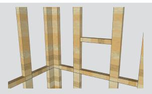
Step 1: Measure the niche and add framing or nogging around the flange area of the niche in the wall frame.
