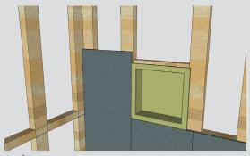
Step 3: Install wallboard to finish flush with outside edge of wall niche flange according to industry standards. (You may need to pack out the wall niche to meet flush with the thickness of the wall lining).
