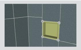
Step 6: Apply AP1000 Aquamox waterproof tape over all screw heads & wall board/niches joins.
